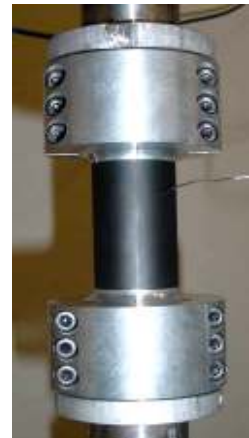
Figure 1: Experimental device for tension-compression, torsion and combined fatigue tests on pipes
