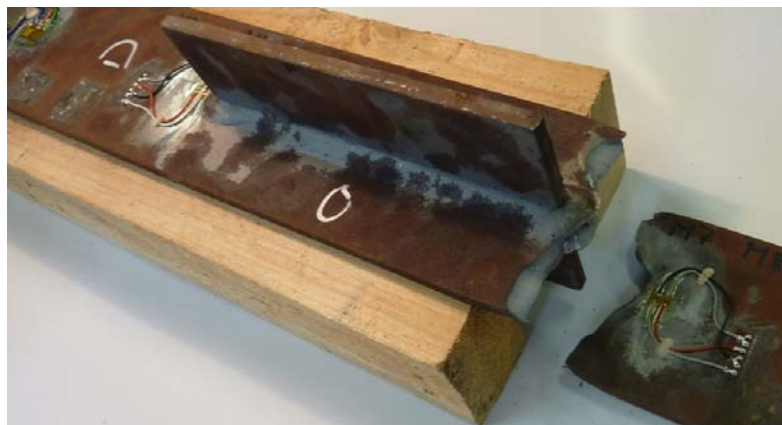
Specimen with longitudinal stiffener L = 200 \text{ mm} ( t = 8 \text{ mm} , S960QL, \Delta\sigma = 495 \text{ MPa} , N_f = 14.580 )
