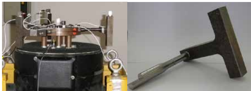
Figure 3: Test bench with specimens in a multiaxial configuration
