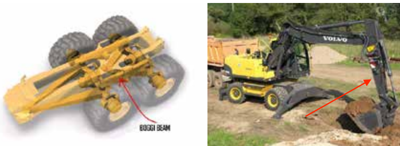
Figure 1 The bogie beam (left) and excavator arm (right).
